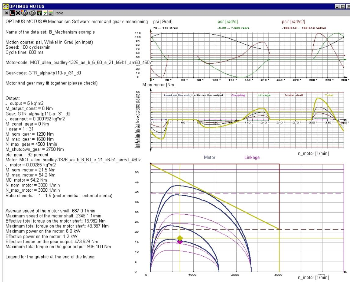
**CAD-OPTIMUS MOTUS ® considers the changing ratios of loads on the controller very precisely! Simple concept tools of the producers of servo controllers have to simplify the calculation that for, that there can be done no reliable design.**
