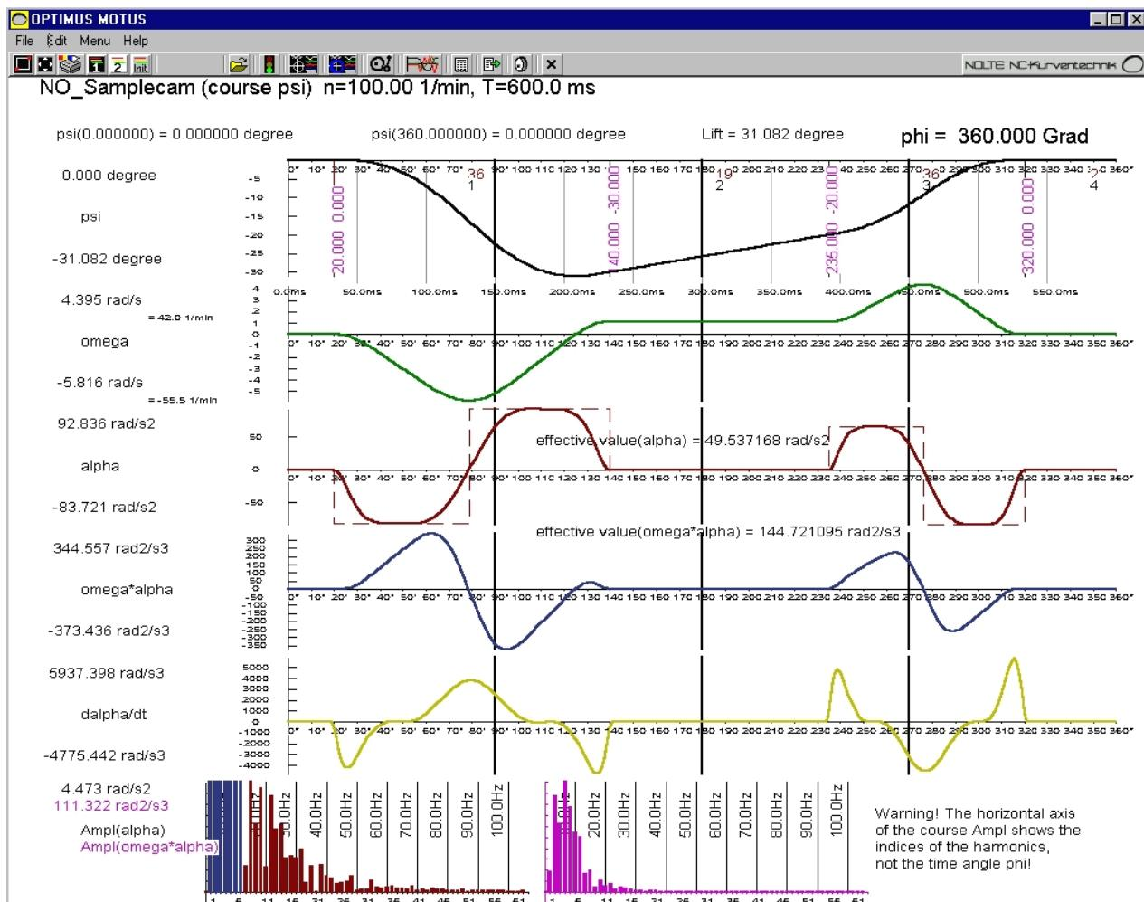
**Optimize the paths of motion with the help of expressive diagrams to deal with following conditions: minimization of vibration, high static loads, high masses, adjustment of internal slack, cutter interference**
